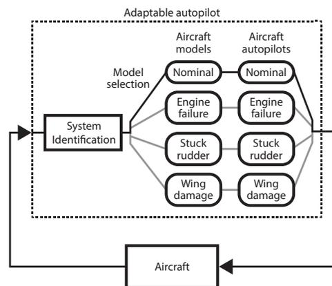
Fig. 5. Overview of the autopilot during its operation. The autopilot continuously identifies the aircraft model and compares it with models from its database. It selects the closest model and applies the autopilot created for that model.
